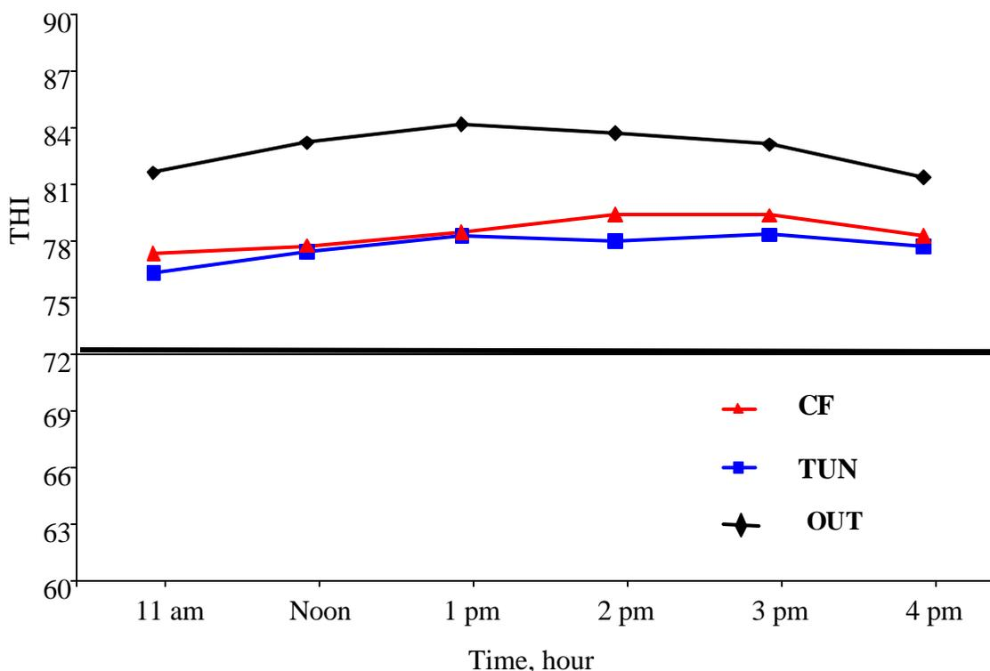
**Figure 4.** 64-day average values of THI for each treatment. TUN- sprinkler cooling with tunnel ventilation; CF- sprinkler cooling with ceiling fans; OUT- outside.
