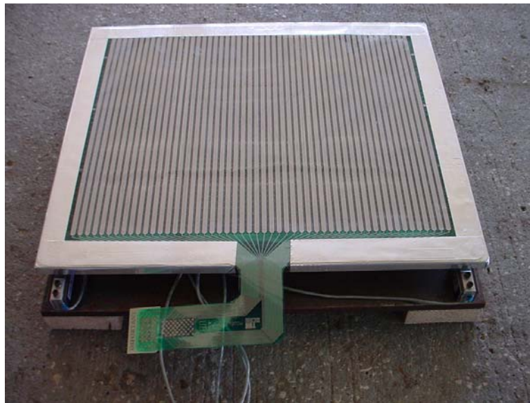
Figure 1. Tekscan Matscan thin pressure measurement film.
